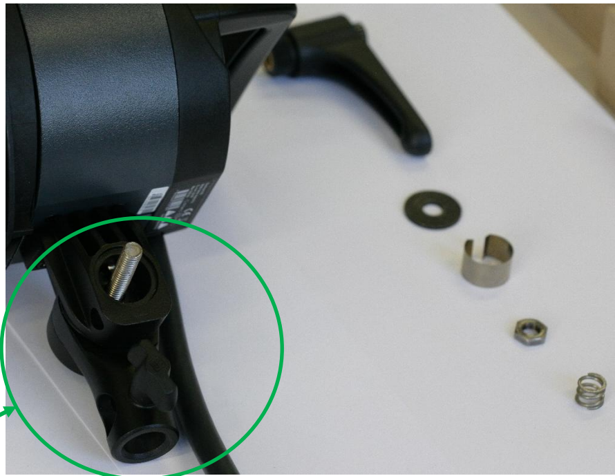
Fig.11: Step 9: Assemble the “moving bracket”, the “custom screw” and the new washer with the “tilt base”.
