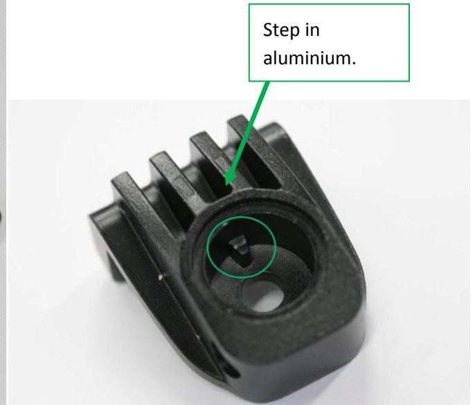
Fig.13: Step 11: After adding Loctite 243 on the thread, Re-mount the nut BN123 M8 and tight up until you are against the step in aluminium.
