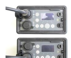
5. Remove the rubber and the housing of the unit.
