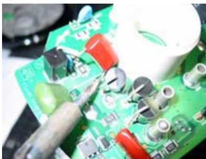
3. now unsolder the second pin and remove the capacitor
