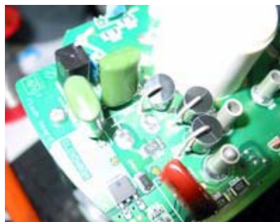
4. assemble / solder the new capacitor from the top side!
