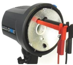
5. Remove the dish reflector and discharge the flash capacitor (HTD voltage) on the flashboard sockets X405, X406
