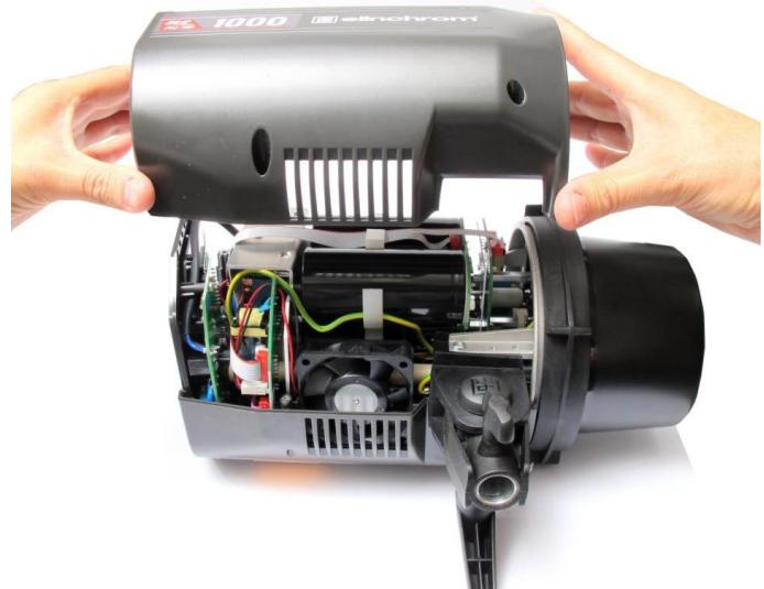
9. Check that the two sides are correctly closed and no wires or cables are stranded between the two housing parts
